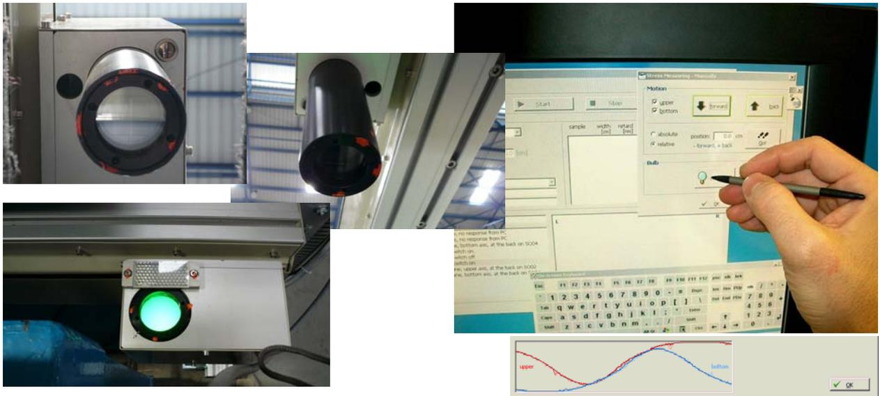
*Stresstter 6™ is a modern machine for automatic off-line non-contact and non-destructive stress measuring in the sheet glass. Stress is measured in several spots across the width of the sheet. Measured stress vector has the orientation of the flowing glass on the production line. Stresstter 6™ is designed to operate with sheet glass of these parameters: length of 1200 to 6000 mm, thickness of 1.6 to 20 mm and width of 1200 to 5600 mm.*
