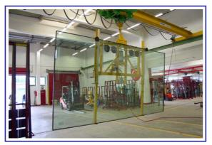
The Venturi device 7005-AB is used to supply the insulation glass unit with large glass panes; the device is used otherwise in the manual cutting unit for feeding the cutting table with glass. Depending upon design, this type of device up can transport up to 1200 kg and sized up to 6.0 x 3.2 m. The extendable side tubes help when adapting to the glass dimensions. If required, these support tubes can also manufactured in such a way that they can be removed.
