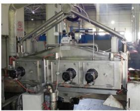
GlassChem HECSt 1800 hot end coating system has been developed specifically for high speed production lines.
