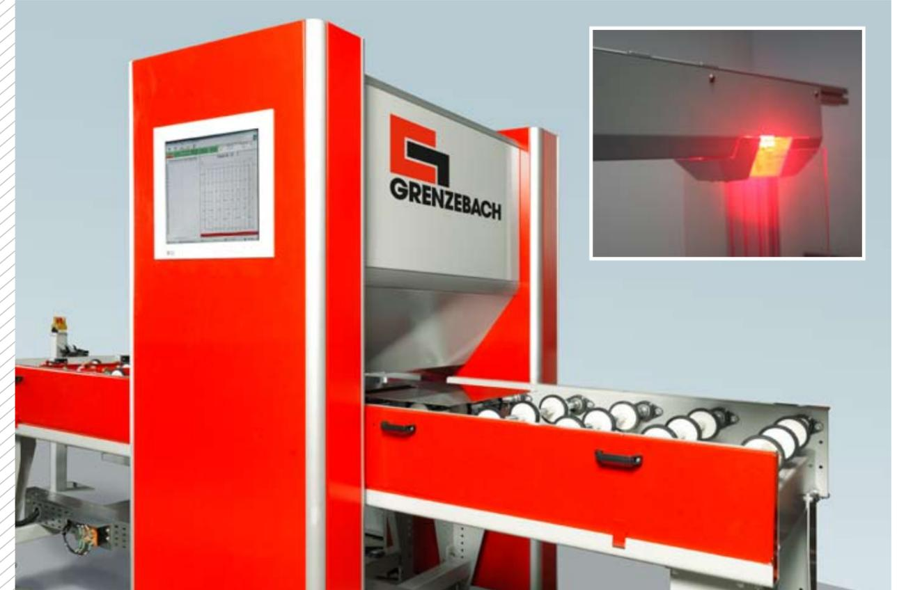
**Glass panels leaving cutting lines** have to be inspected especially for the correct sizes, rectangularity and edge damage.
