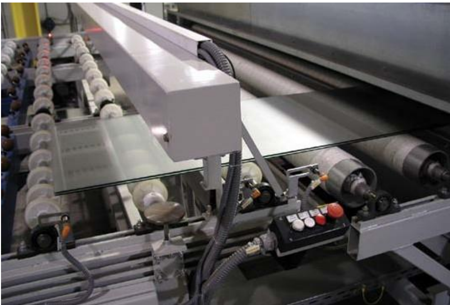
Precise nip control keeps layers aligned during de-airing
