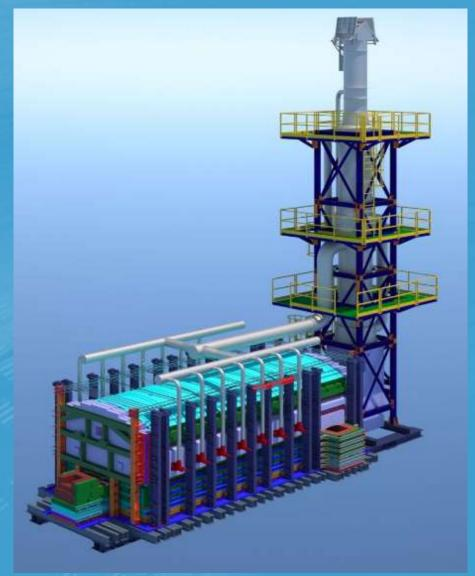
The recuperative melting furnace is a sophisticated apparatus which requires a relatively low budget compared with a regenerative furnace of same size.
