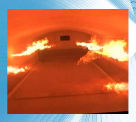
FALORNI TECH has the right burner for each furnace and for each glass melting process. Our burners are designed in full integration with the combustion system and the furnace geometry. All our burners can fire varied types of fuel depending on availability (NG, LPG, Propane, HFO, LFO). Our family includes also Oxy-fuel burners
