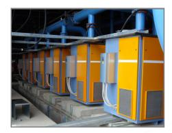
The systematic replacement of water cooled pumps with Pneumofore UV50 units at HNG involved in 2012 the Naidupeta and Nashik plants, where a new logic was installed, combined with a Variable Speed drive and an Eternet card for each vacuum pump.
