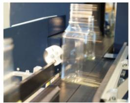
Allocators are integral parts of inline-sorting, above all, in bottling plants and the food and drink industry. Due to the high production speed, modern systems work with powerful control systems, highly dynamic drive technology and precise industrial image processing. We have developed our own Allocator based on our comprehensive know-how of the container glass manufacturing process. This combines image processing, SPS and servo-motor drive technology into a compact and easy to integrate unit.
